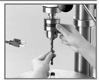
Figure 32. Installing bit.
